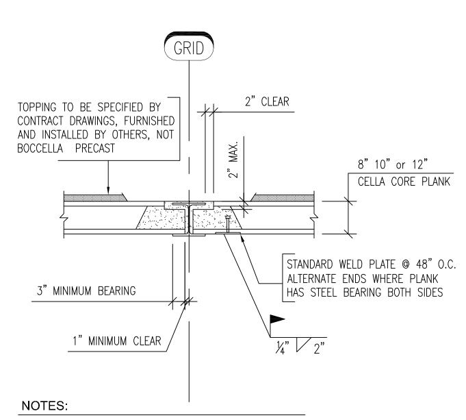
IT IS STANDARD INDUSTRY PRACTICE TO ONLY WELD ONE END OF A PIECE OF HOLLOWCORE PLANK. WELDING BOTH ENDS OF A PLANK WILL RESULT IN VOLUME CHANGE RESTRAINT FORCES THAT MUST BE CONSIDERED IN THE DESIGN OF THE CONNECTION. IF WELD PLATES MUST BE USED, BOCCELLA PRECAST RECOMMENDS WELDING ALTERNATE ENDS OF THE PLANK, OTHERWISE THE ENGINEER OF RECORD IS TO PROVIDE ALL FORCES FOR CONNECTION DESIGN.
